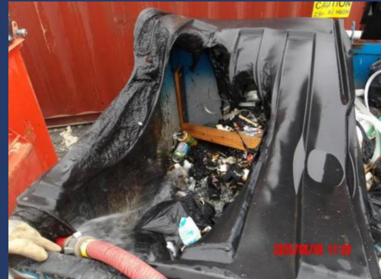
Burnt interior of the waste bin with multiple discarded vape pens
